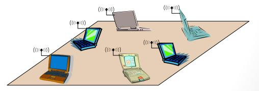
→ A wireless ad hoc network (WANET) is a decentralized type of wireless network that does not rely on a pre existing infrastructure.
